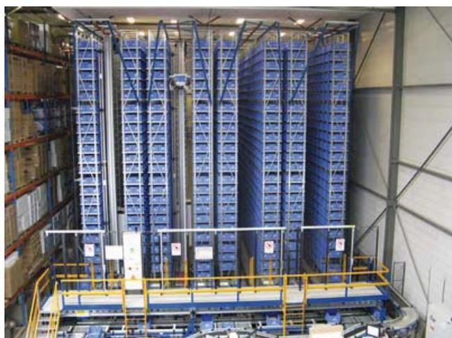
**The Mini-load system at Highlite's headquarters. This fully-automated picking system comprises four cranes and 40,000 bins in a goods-to-man principle, with a maximum pick capacity of 500 picks/hour.**
